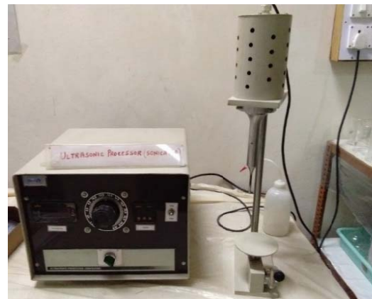
Figure 5: Sonochemical process for growth of nanoparticles using Horn type Ultrasonicator, available at RLES, Department of Physics, NSIT
